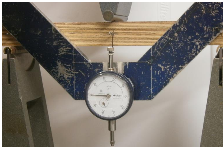
Figure 3 - Typical Yoke and Dial Gauge Assembly
