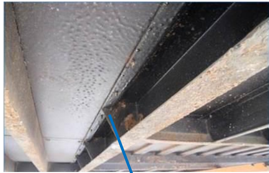
Tunnel bolster Gusset RLG
