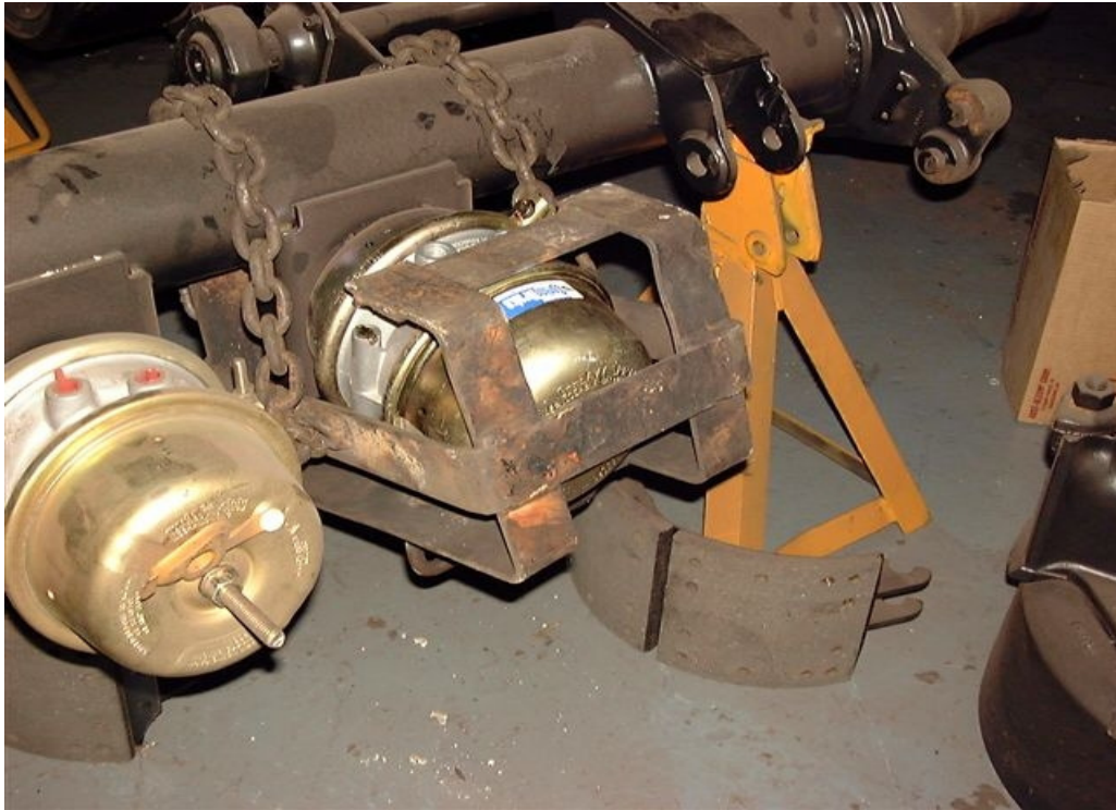
(Brake chamber locked inside safety chamber)
