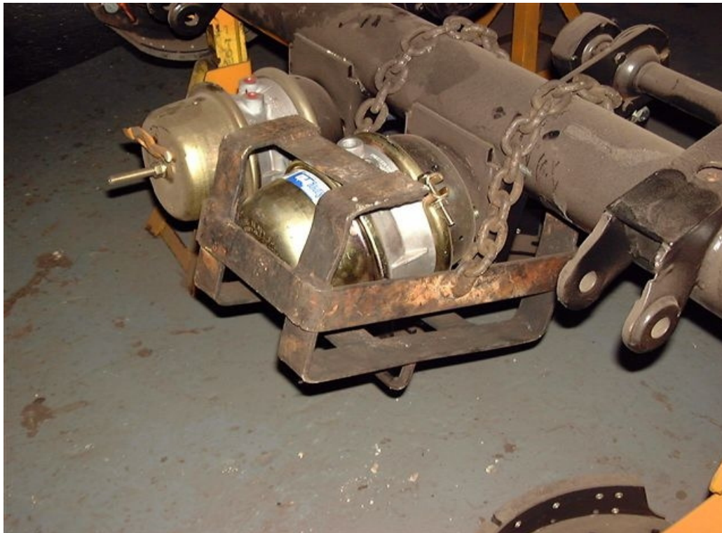
(Brake chamber locked inside safety chamber)
