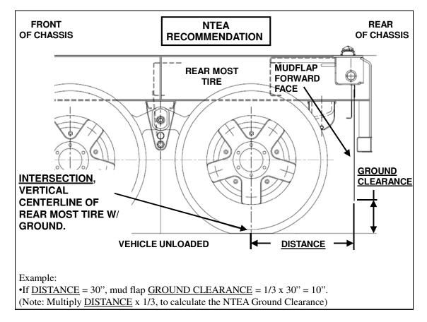
It should be noted that the NTEA recommendation locates the bottom edge of the flap closer to the ground. In lieu of any State rule which requires still less distance, this may be preferred by owners/operators.
