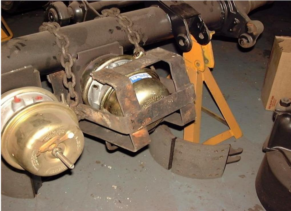
*(Brake chamber locked inside safety chamber)*
