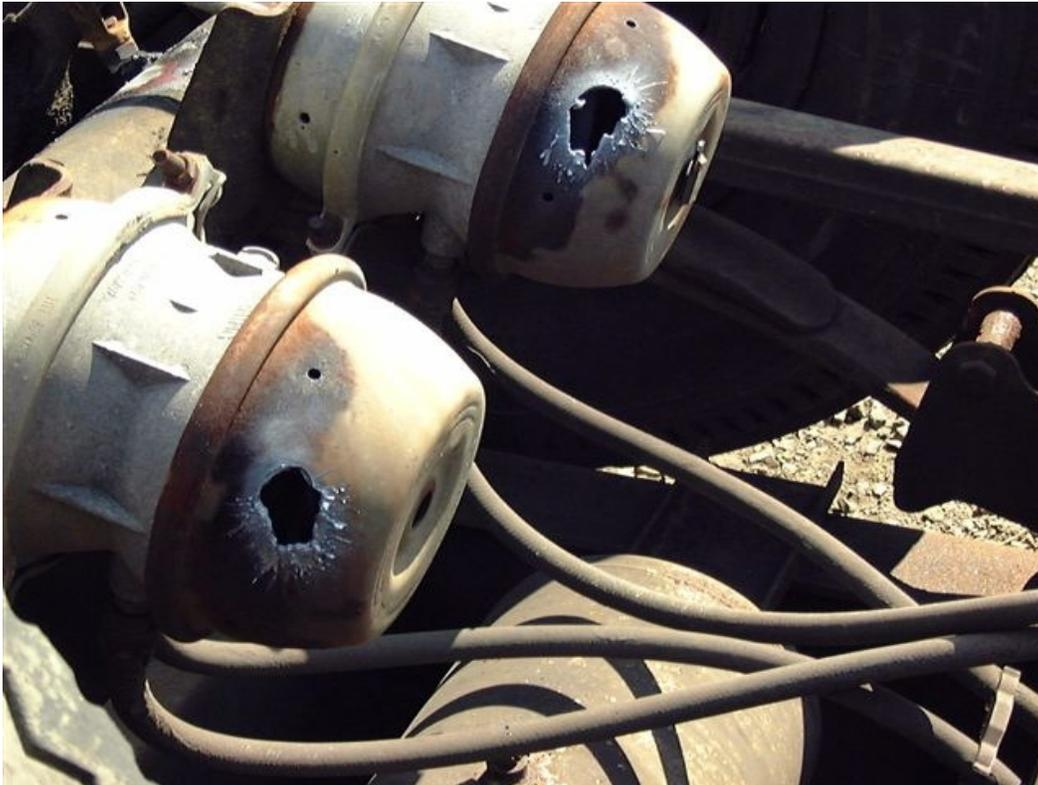
*(Cut holes through brake chamber head housing and spring)*
