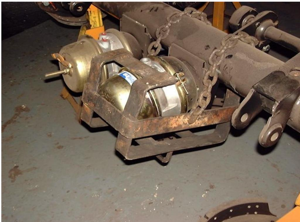
*(Brake chamber locked inside safety chamber)*
