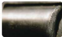
Roller end wear
