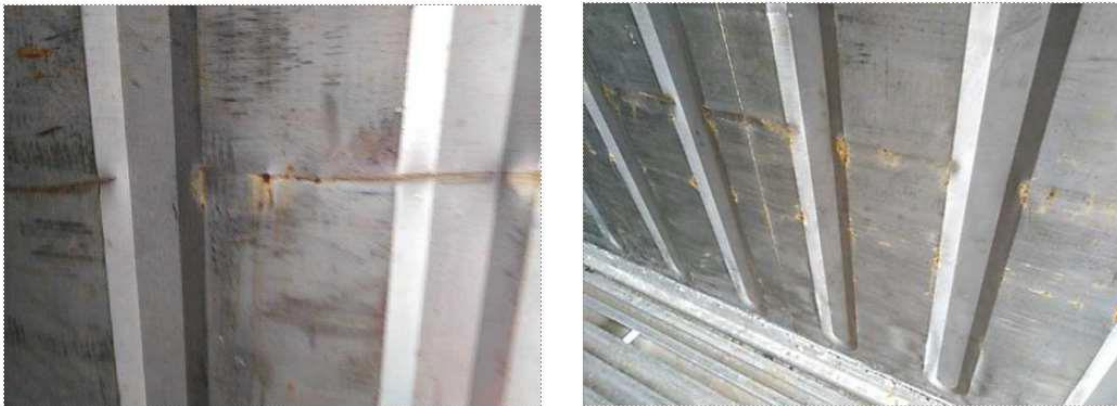
Minor rusty scratches on the HGSS panels due to loading/unloading operations, Refer to IICL General Guide for Container Cleaning, 3rd Ed.
