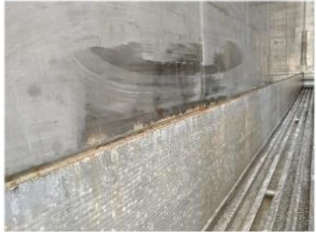
Scuff liner and aluminum T-floor showing oxidation and corrosion as result of chemicals spraying. Repair required.
