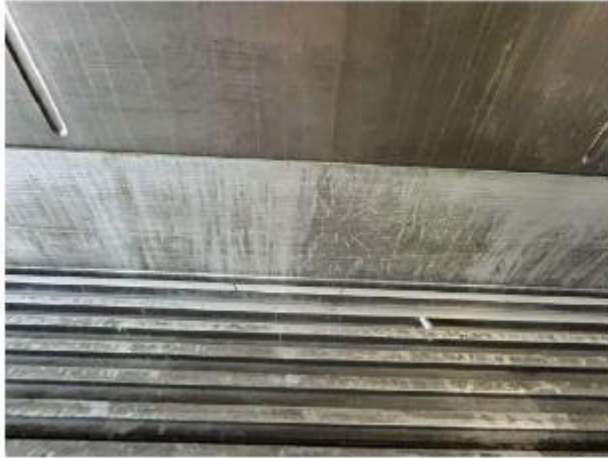
Scuff liner and aluminum T-floor showing oxidation and corrosion as result of chemicals spraying. Repair required.
