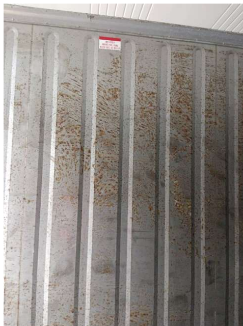
Contaminated panels showing rust/corrosion marks spread over large areas including weld seams, corrugated and flat surfaces. Above photos depict typical damage caused by contamination as result of chemical spraying. Repair required.
