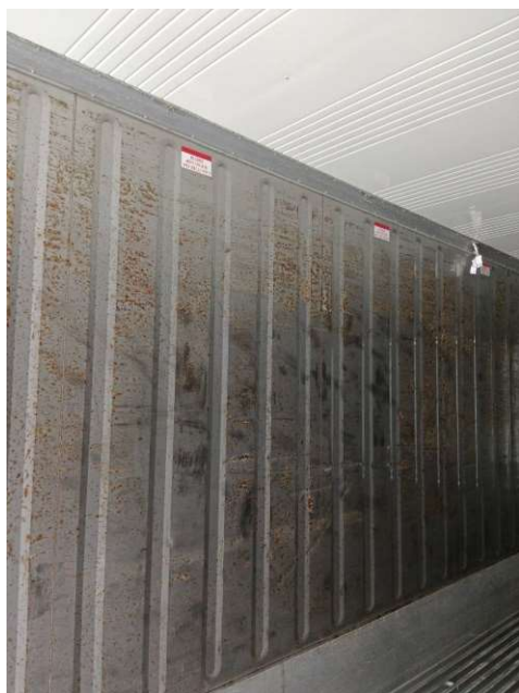
Contaminated panels showing rust/corrosion marks spread over large areas including weld seams, corrugated and flat surfaces. Above photos depict typical damage caused by contamination as result of chemical spraying. Repair required.
