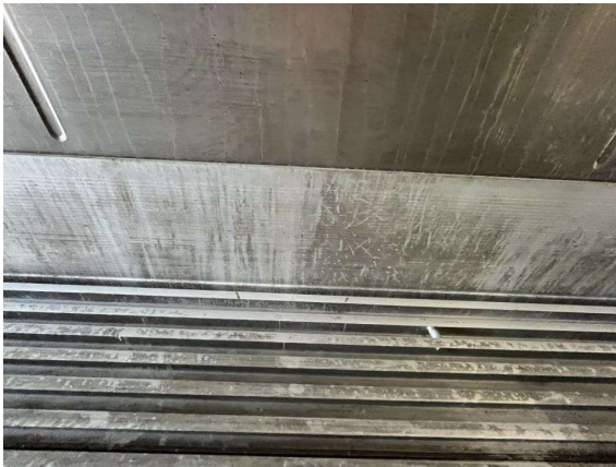
Scuff liner and aluminium T-floor showing oxidation and corrosion as result of chemicals spraying. Repair required.
