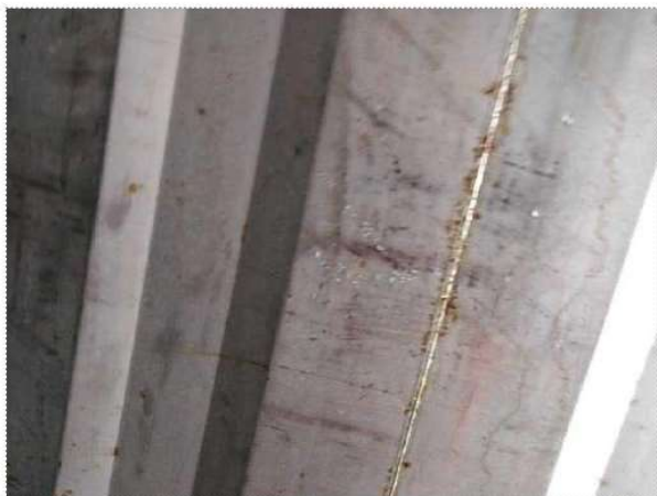
Superficial rust near the welding seam area, Refer to IICL General Guide for Container Cleaning, 3rd Ed.
