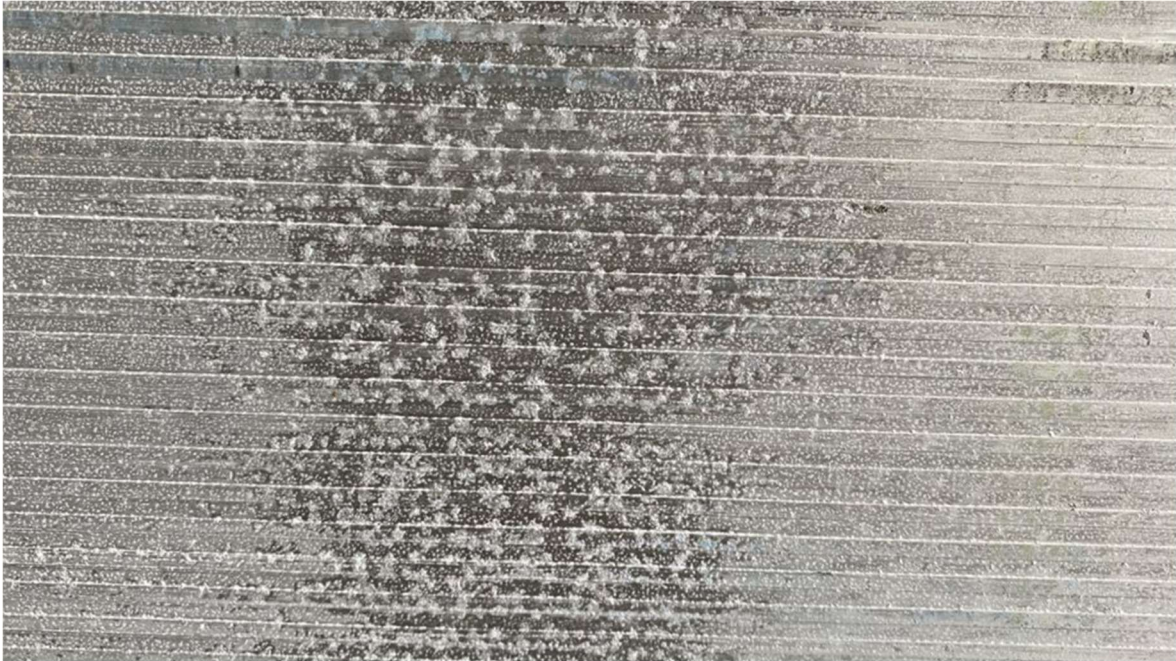
Contaminated pitting on scuff liner. Repair required.
