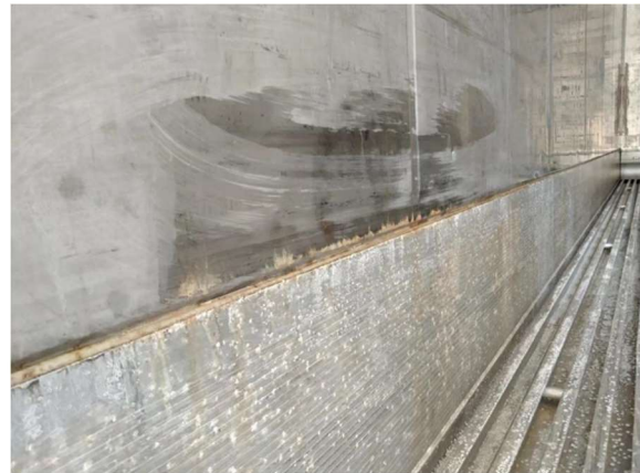
Scuff liner and aluminium T-floor showing oxidation and corrosion as result of chemicals spraying. Repair required.
