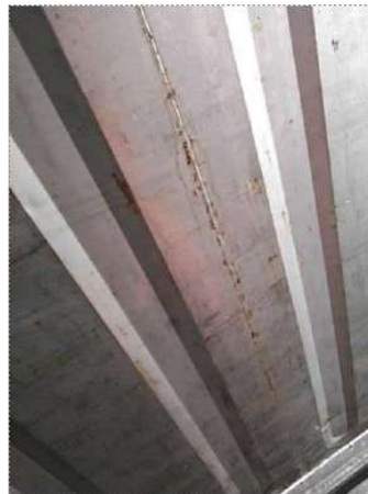
Superficial rust near the welding seam area, Refer to IICL General Guide for Container Cleaning, 3rd Ed.
