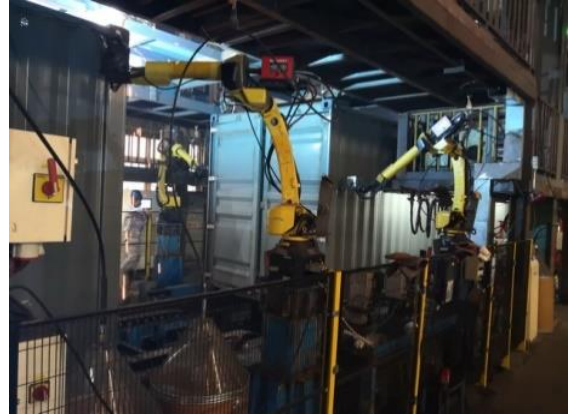
Continuous weld between side panels and corner posts
