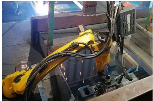
Roof corner reinforcement plate being welded to header and extension plate
