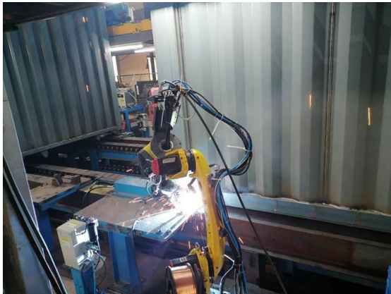
Corner reinforcement plate being welded to the bottom side rail
