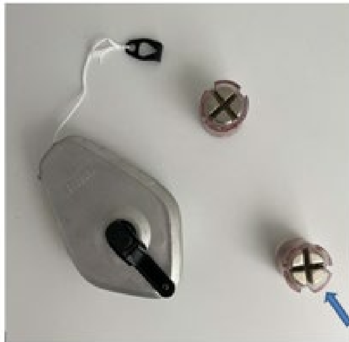
Magnets are now encased in plastic to reduce chances of chipping.
