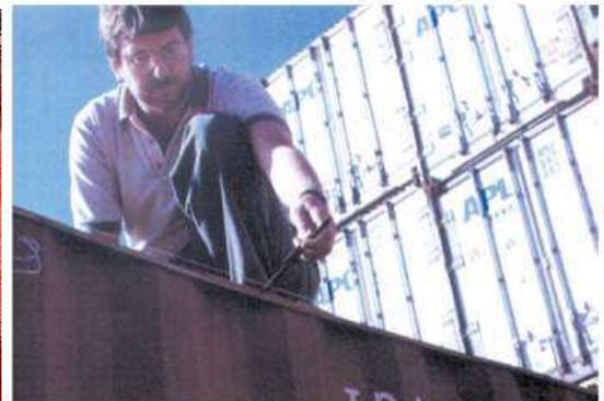
Measuring bows to rails: the inspector measures distance from reference line to point of maximum deflection in a flat-bar top side rail. In the case of bows, the reference line must be extended across the full length of the rail. See Section 4.2.3.
