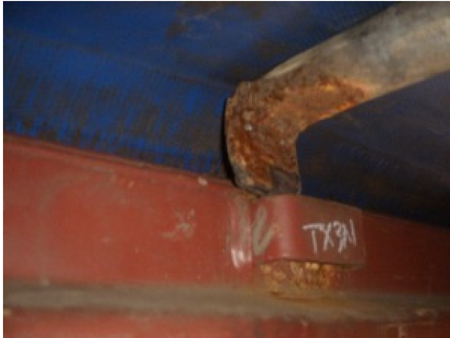
Improperly fitted roof bow end
